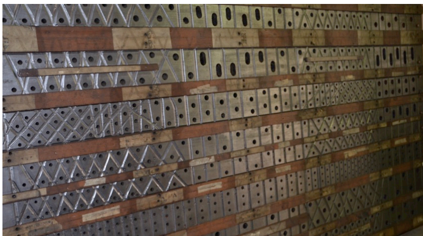
The swell table with bearers in place showing the slideways for the stop sliders
